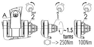
To adjust the brake of the link, following actions have to be done:
